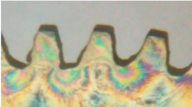
Fig 4. Fringe Pattern at the Tooth Root
