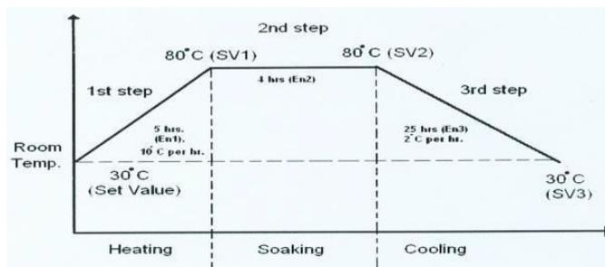
Fig 3. Stress Freezing Cycle
